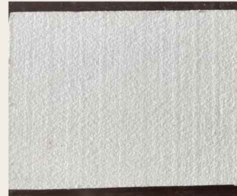
Colour Fading Testing (After 4 month exposure)
