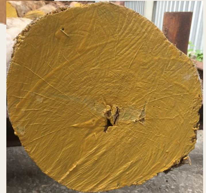
With Log Sealant
